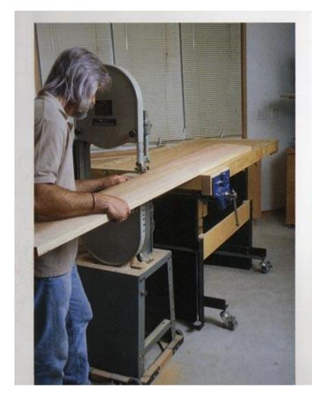
■ INSTANT OUTFEED. You can raise a workbench to catch the ends of long, heavy boards as they come off the bandsaw, making sawing more accurate and less tiring. The ADJUSTABENCH® in Geoffrey Noden's shop features a range of bench heights to accommodate various setups, with locking casters that keep it steady as you saw.
