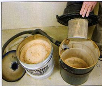
Oneida's Dust Deputy is a cyclone powered by a shop vacuum. The cyclone separates the dust and dirt, which drop into the Oneida dust drum, while the air exhausts through the vac and its filter back into the shop.
