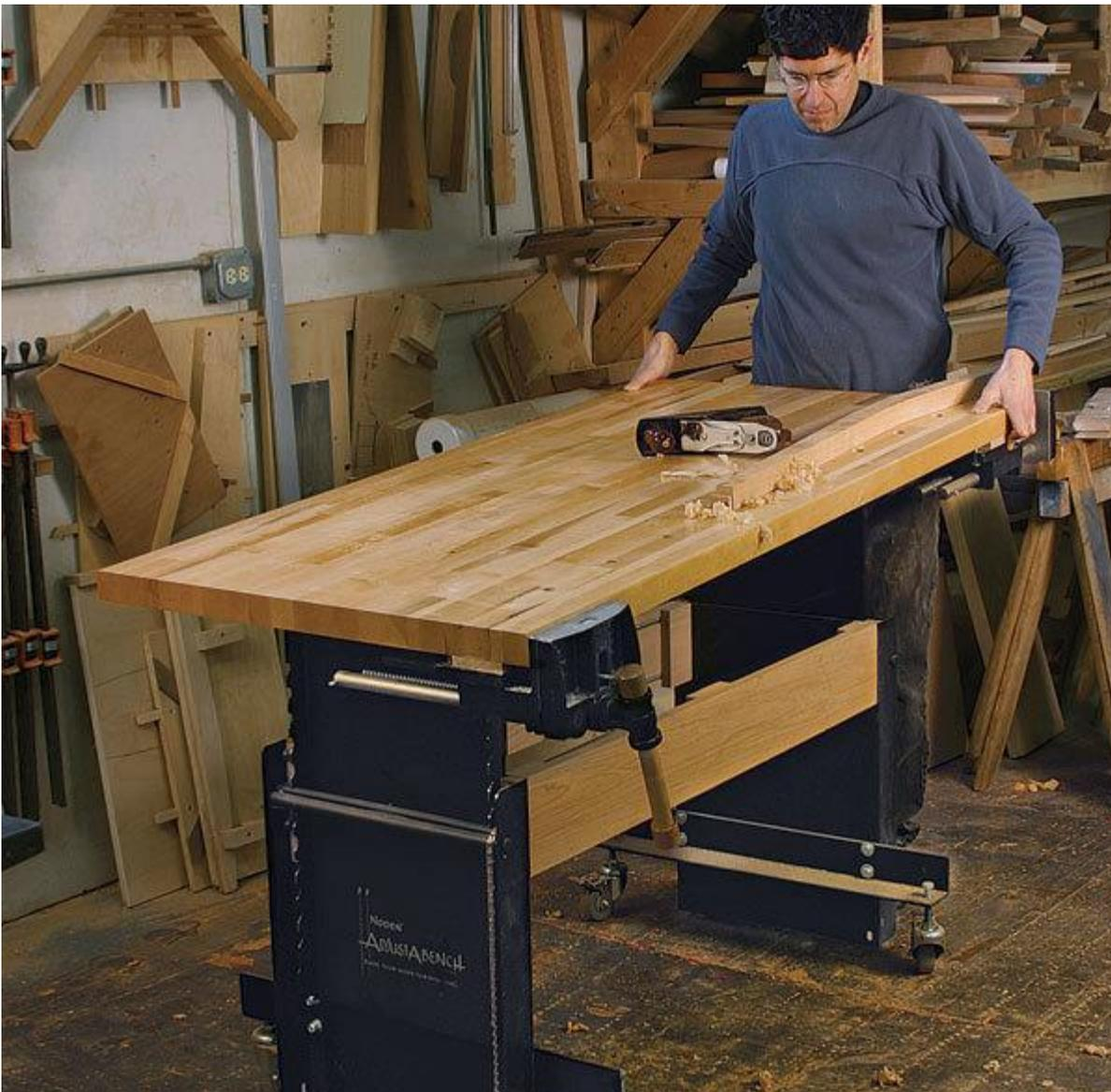
I'm a big advocate of working at the proper height for specific tasks. So I was intrigued by the concept of the Noden Adjust-a Bench, a workbench system that can be adjusted to a variety of heights.
