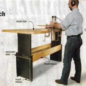
It's easy to raise the top, Just lift it, one end at a time. The ratcheted adjustment system has twelve stops. Stepping on the foot pedal while lifting up on the top releases the ratchet and lowers the top. Accidentally stepping on the pedal while you're working won't make the top come crashing down.
